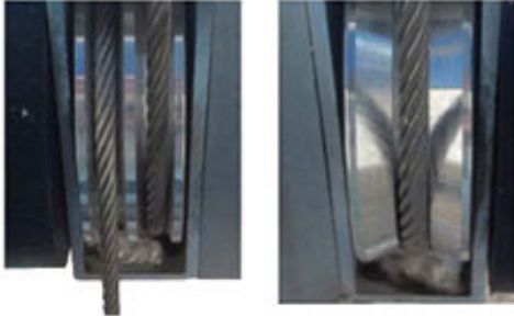
The "V" shaped aluminum pulleys with brass oilite bushing riding on a stainless steel, greasable pins with stainless cables are designed for years of trouble free use.
